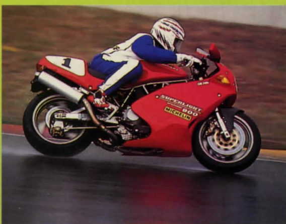
Despite a third less horsepower than the 888, the Superlight could stay with it in the wet due to its brilliant centre of gravity and low-down torque
