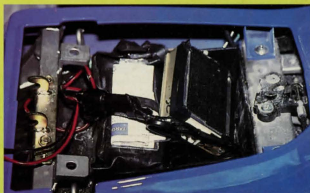
...the digital transponders were fitted to each bike, in this case under the seat...
