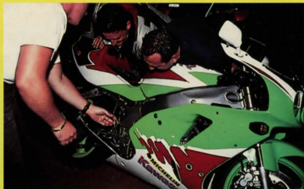
The equipment being fitted to this ill fated ZXR is part of Mugello's advanced digital timing system. Around the circuit there are 30 ish pick up points that register every time a bike fitted with a transponder passes...
